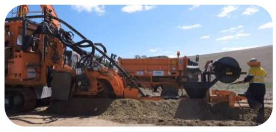
The laying box, installs all the cables, TR sand, hard cover, screened backfill and warning tape, all in only one pass, without any obstacle between the drum and the bottom of the trench which guarantees the cables installation integrity.
