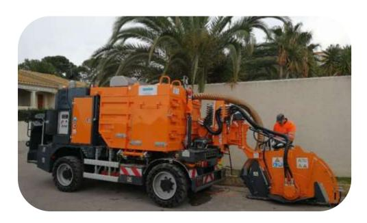
The mini-Cleanfast combines both SideCut and CleanFast advantages for an efficient micro trenching in the tightest environments
